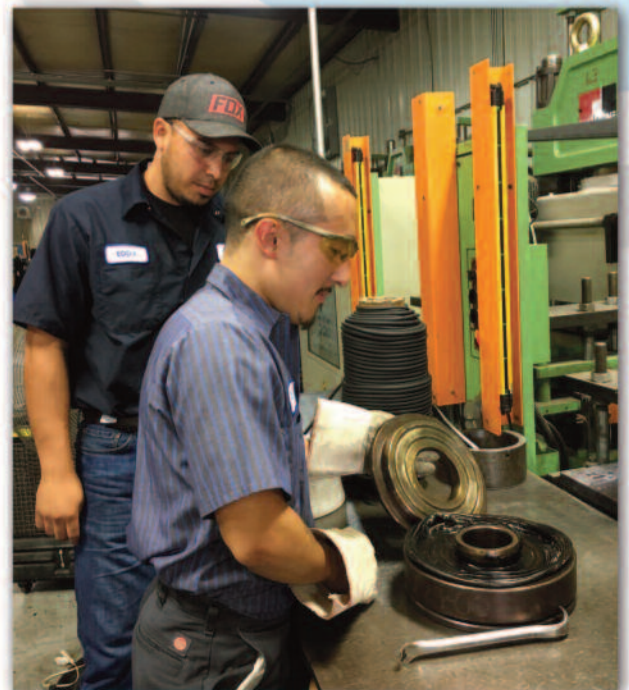
72 compression molding presses and two rubber extruders which pre-form elastomeric shapes prior to final molding
